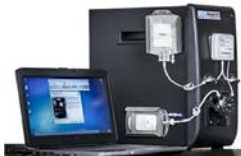
Figure 2. MaxCyte® STX electroporation transfection apparatus. Pictured is the apparatus set up for 100mL flow electroporation and expansion to a 4L culture. The experiments described here utilized the 0.4mL cuvette and 15mL culture volumes.
